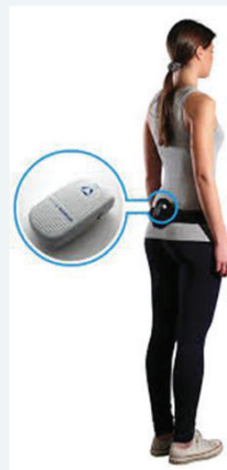
Figure 2: BTS G-Walk sensor body positioning on spinal L5.
