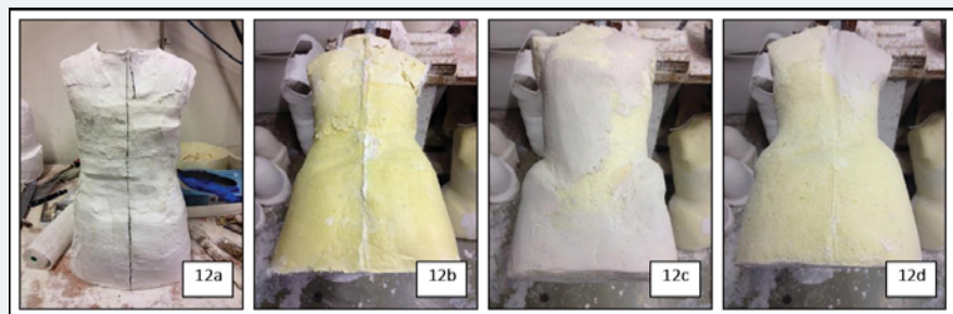
Figure 12a-d: Pedilen device mould starting from the plaster cast (own elaboration).
