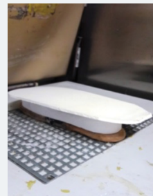
Figure 11: Plaster placement in the vacuum before the EVA thermoforming (from own elaboration).
