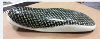
Figure 17: Carbon-kevlar shell after thermoforming (from own elaboration).
