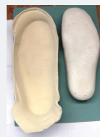
Figure 13: Result of thermoforming of EVA and plaster cast (from own elaboration).
