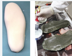
Figure 14: Thermoformed EVA on plaster cast and positioning of the first layer in kevlar-carbon (from own elaboration).
