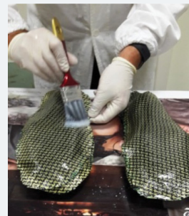
Figure 15: Application of the resin after the second application of the kevlar-carbon layer (from own elaboration).
