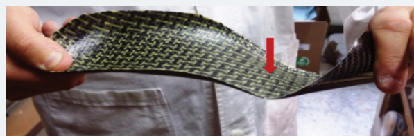
Figure 19: Carbon shell only with indication of the torsion wing at the head of the metatarsal head and of the structural elasticity in torsion of the body (from own elaboration).
